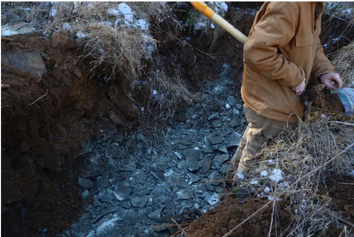
Photo 5. Shallow bedrock, shown here in Test Pit 1. Greenish-gray sandstone in nearly flat beds.
