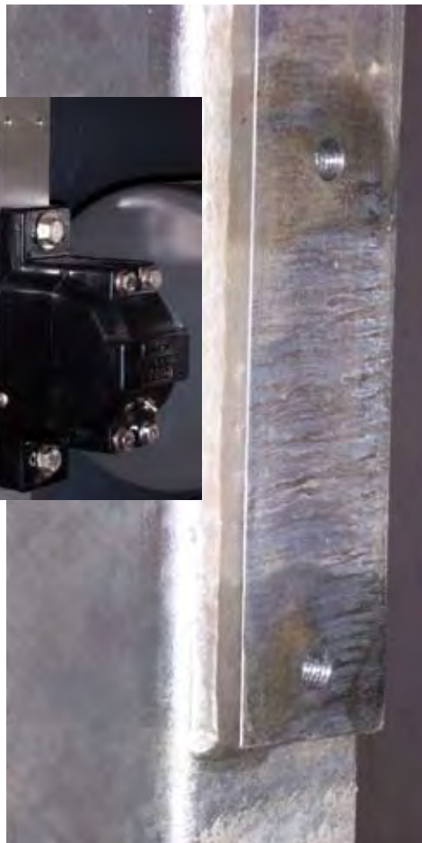
Machined Mounting Pads/Tubular Steel Frame
