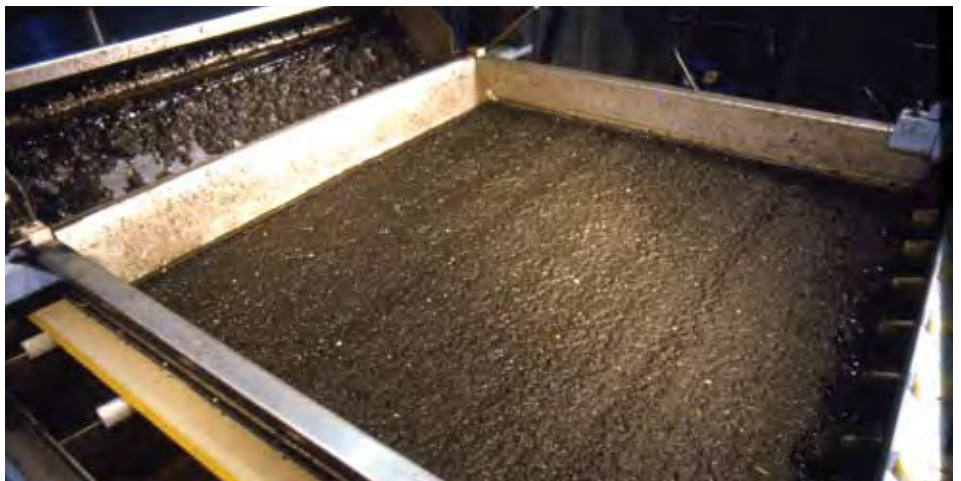
Uniform slurry distribution
